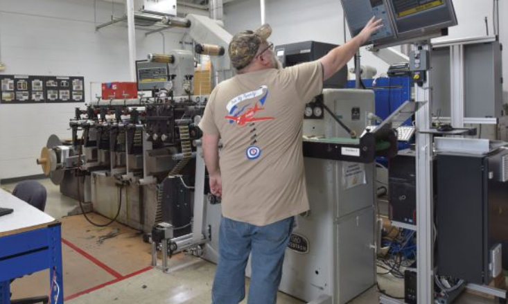
Mike Brownrigg runs a job on one of Argent Tape & Label's six flexographic presses.
